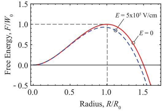
FIG. 1. Free energy of a spherical cavity in a metal. A slight lowering of the barrier requires  $E = 4 \times 10^5$  V/cm at the plasmon frequency of  $\omega_r = \sqrt{2/3} \omega_p$ . Parameters values are typical for void nucleation in metals (see, e.g., Ref. 11):  $\sigma = 1$  J/m<sup>2</sup>,  $R_0 = 0.5$  nm,  $W_0 = 1$  eV,  $\omega_p = 10^{15}$  rad/s, and  $\tau = 10^{-12}$  s, with  $\epsilon_p = 1$ .
