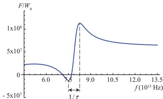
FIG. 3. Normalized free energy of an oblate spheroidal cavity vs. field frequency  $f = \omega/2\pi$ , with  $E = 3 \times 10^3$  V/cm. The sharp resonance of width  $1/\tau$  determines the aspect ratio  $R_\parallel/R_\perp \approx (\omega/\omega_p)^2 \approx 10^{-4}$ . Numerical values are the same as those used in Fig. 1.
