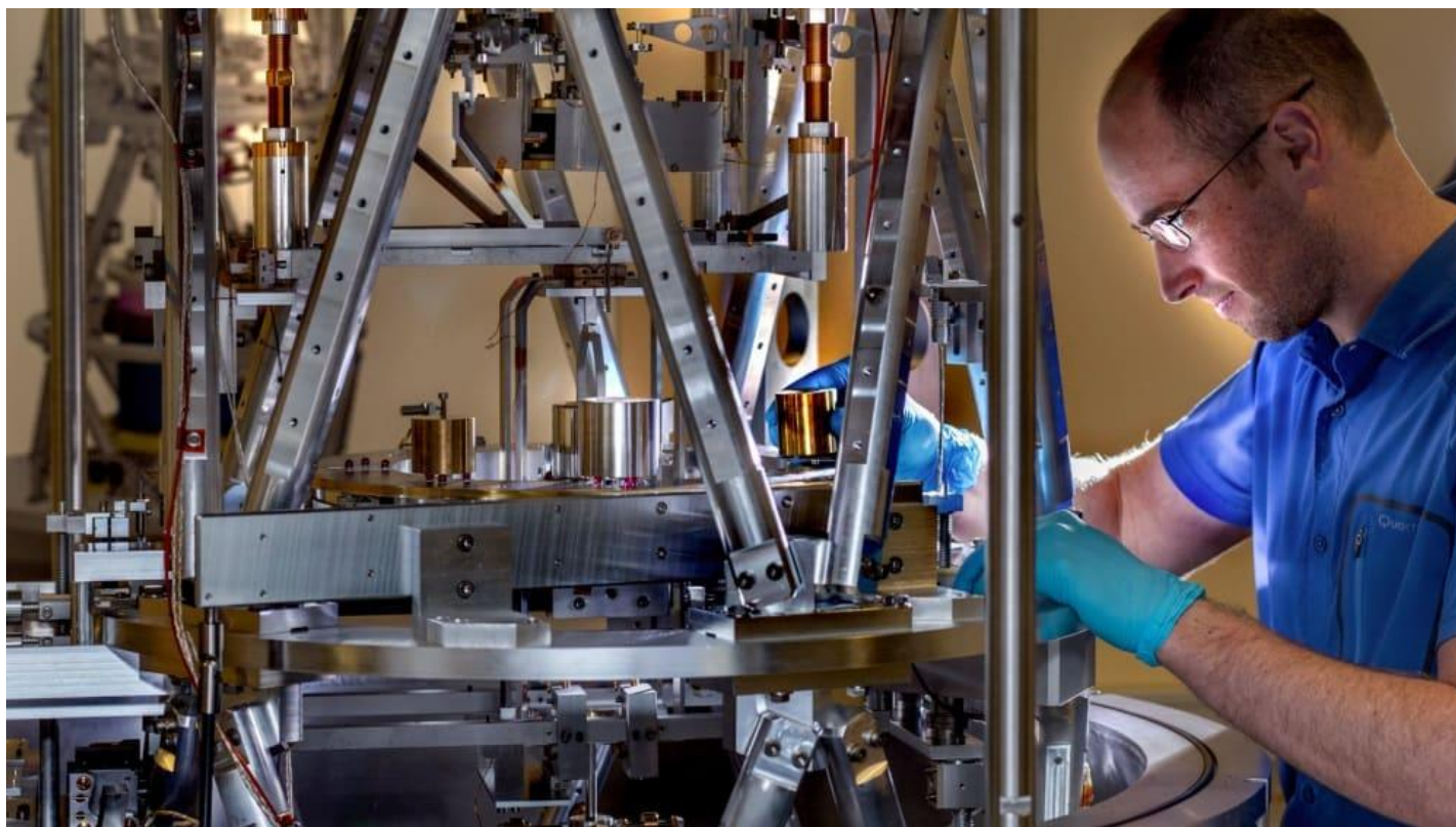
All change: work on the redefinition of the kilogram was carried out using a Kibble balance. (Courtesy: BIPM)
