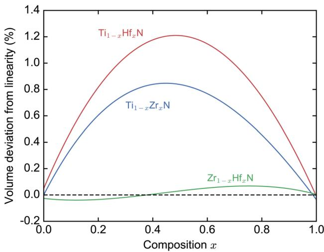
**Figure 5.** Volume deviations from linearity of  $\text{Ti}_{1-x}\text{Zr}_x\text{N}$ ,  $\text{Ti}_{1-x}\text{Hf}_x\text{N}$  and  $\text{Zr}_{1-x}\text{Hf}_x\text{N}$ . Curves indicate CE-fitted values of the random solid solution configurations.
