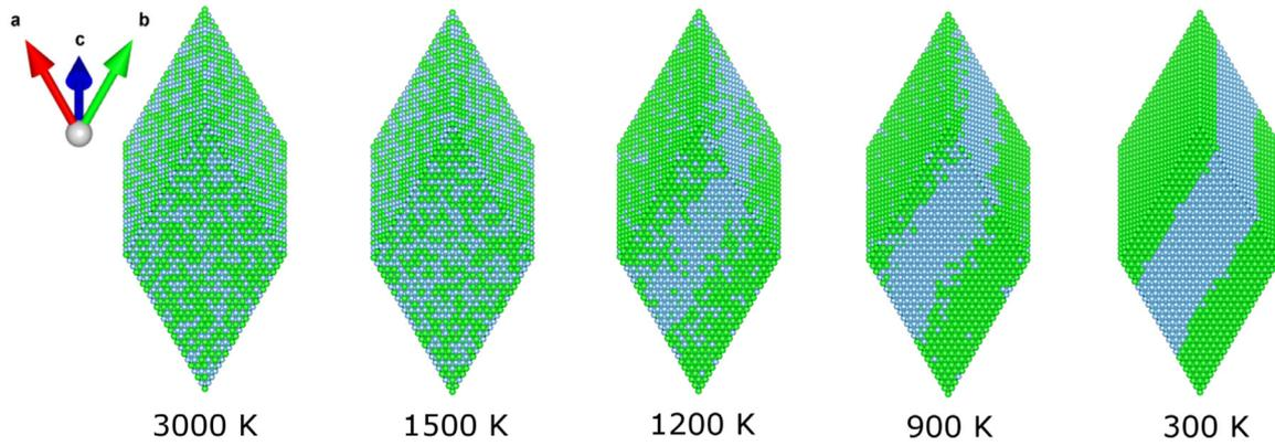
**Figure 4.** Monte Carlo simulation cells of  $\text{Ti}_{0.5}\text{Zr}_{0.5}\text{N}$  at 3000 K (far above the miscibility gap), 1500 K (just above the miscibility gap 1400 K), 1200 K, 900 K and 300 K (within miscibility gap). Blue and green balls are Ti and Zr atoms. N atoms are omitted from the display for clarity. Increasing tendency towards separation is clearly visible with lowering temperature.
