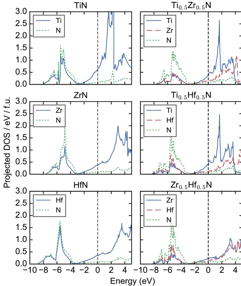
**Figure 2.** Projected density of states of TiN, ZrN, HfN and three solid solutions with composition  $A_{0.5}B_{0.5}N$  where A and B are transition metals. The Fermi energy is set to 0.
