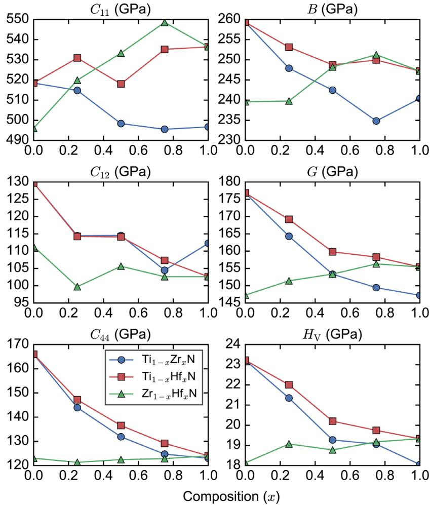
**Figure 7.** Elastic constants  $C_{11}$ ,  $C_{12}$ ,  $C_{44}$ , bulk moduli ( $B$ ), shear moduli ( $G$ ) and Vickers hardness ( $H_V$ ) of the SQS's of  $\text{Ti}_{1-x}\text{Zr}_x\text{N}$ ,  $\text{Ti}_{1-x}\text{Hf}_x\text{N}$  and  $\text{Zr}_{1-x}\text{Hf}_x\text{N}$ . Lines are a guide to the eye.
