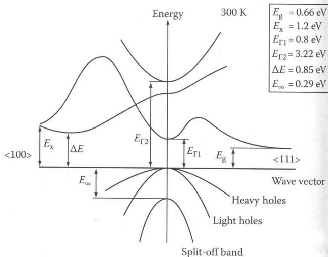
**FIGURE 16.8** Band gaps in bulk Ge. (Adapted from Yu, B. et al., *J. Clust. Sci.*, 17, 579, 2006.)
