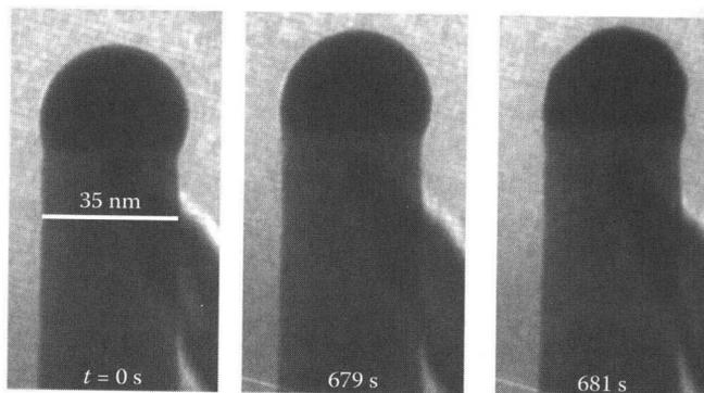
**FIGURE 16.6** Representative bright-field TEM image series showing the solidification of AuGe catalyst on top of a Ge wire when the  $\text{Ge}_2\text{H}_6$  pressure is reduced during growth at a constant temperature  $T = 340^\circ\text{C}$ . In this experiment,  $\text{Ge}_2\text{H}_6$  pressure was dropped from  $1.1 \times 10^{-6}$  Torr to  $2.8 \times 10^{-7}$  Torr at  $t = 0$ . (Adapted from Kodambaka, S., Tersoff, J., Ross, M.C., and Ross, F.M., *Proc. SPIE*, 7224, 72240C, 2009.)
