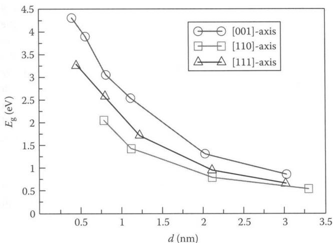
**FIGURE 16.10** Dependence of band gap on the wire diameter and orientation. (Adapted from Medaboina, D. et al., *Phys. Rev. B*, 76, 205327, 2007.)
