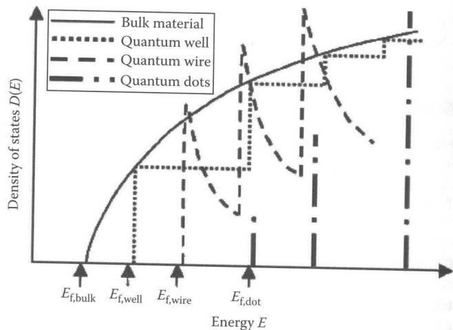
**FIGURE 16.2** Density of states of different nanostructures compared to bulk material. (Adapted from Chen, G. and Shakouri, A., *J. Heat Transfer T ASME*, 124, 242, 2002.)
