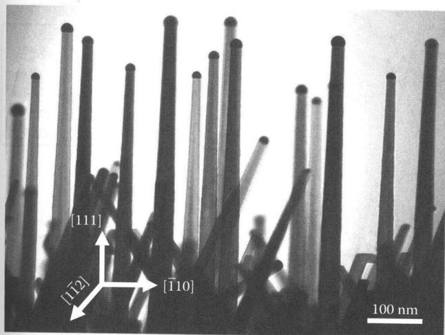
**FIGURE 16.5** A typical bright-field TEM image obtained from a Si(111) sample during the VLS growth of Ge nanowires. Most wires grow epitaxially in the  $\langle 111 \rangle$  direction. (Adapted from Kodambaka, S., Tersoff, J., Ross, M.C., and Ross, F.M., *Proc. SPIE*, 7224, 72240C, 2009.)
