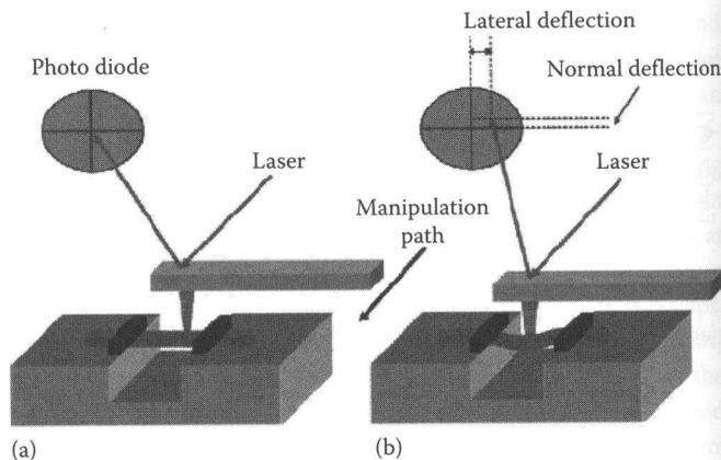
**FIGURE 16.13** Schematic of the lateral nanowire manipulation experiment setup: (a) before manipulation, (b) during manipulation. The nanowire under investigation is suspended over a trench in the substrate and fixed by Pt deposits at the trench edges. During the manipulation the lateral and normal cantilever deflection signals are simultaneously recorded. (Adapted from Heidelberg, A. et al., *Nano Lett.*, 6, 1101, 2006.)
