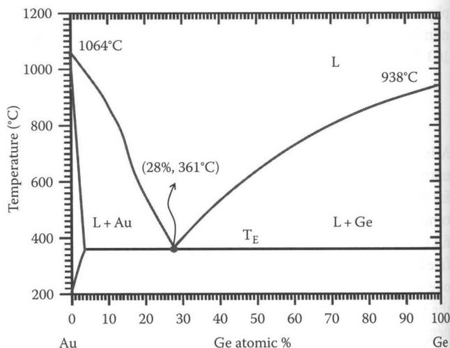
**FIGURE 16.4** Au-Ge phase diagram. (Adapted from Okamoto, H. and Massalski, T.B., *Binary Alloy Phase Diagrams I*, ASM International, Gaithersburg, MD, 1986.)
