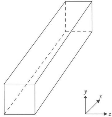
**FIGURE 16.1** Infinitely long rectangular nanowire with the potential inside taken to be  $V = 0$  and outside as infinity. (Adapted from Harrison, P., *Quantum Wells, Wires and Dots*, John Wiley & Sons, West Sussex, U.K., 1999.)
