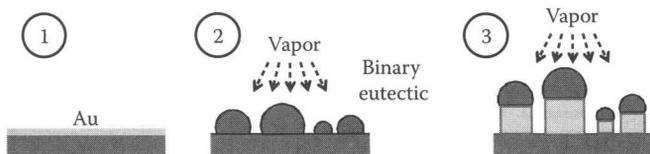
**FIGURE 16.3** Schematic of vapor-liquid-solid process. Au is shown in panel (1), half-circles in panel (2), and (3) at the top of the wires are Au catalysts. Bottom region is the substrate. (Adapted from Kodambaka, S., Tersoff, J., Ross, M.C., and Ross, F.M., *Proc. SPIE*, 7224, 72240C, 2009.)
