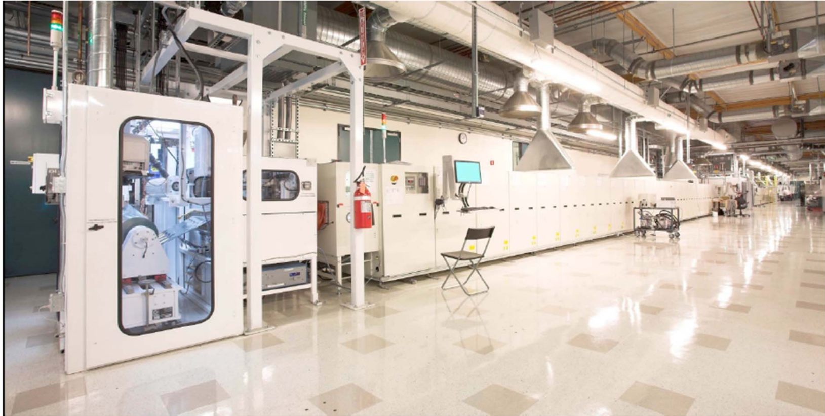
Figure 9: A Nanosolar roll-to-roll processing tool for rapid semiconductor formation, San Jose, California.
