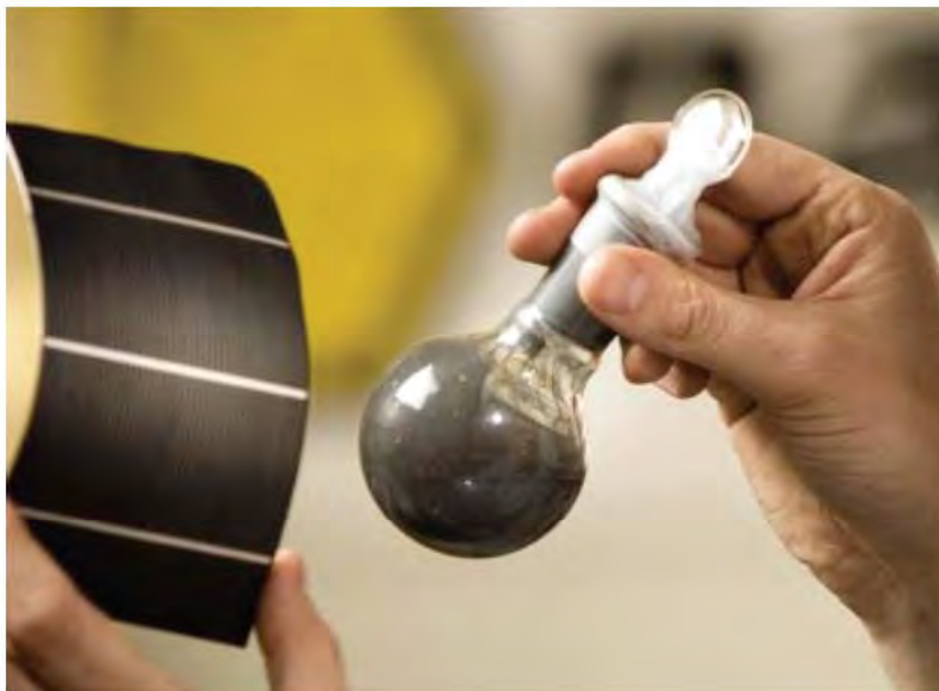
Figure 6 and 7: A laboratory sample of our nanoparticle ink. Nanoparticles shown to the right are an average of 20nm in diameter.
