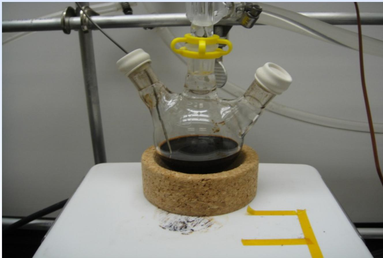
Typical three-headed flask set up. The middle head is connected to the Schlenk line's glass manifold. The left head is covered with a septum pierced by the thermocouple. The right head is for injection. Photo and caption courtesy of T. Kinner (UT).
