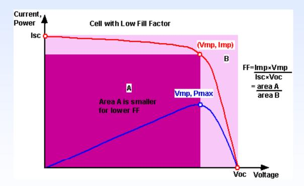
Graph of cell output current (red line) and power (blue line) as function of voltage. Also shown are the cell short-circuit current ( $I_{sc}$ ) and open-circuit voltage ( $V_{oc}$ ) points, as well as the maximum power point ( $V_{mp}$ ,  $I_{mp}$ ). Click on the graph to see how the curve changes for a cell with low FF.
