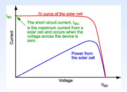
$I_{SC}$  is due to the generation and collection of light-generated carriers. For an ideal PV cell with moderate resistive loss,  $I_{SC}$  and the light-generated current are identical ( $I_{SC}$  is the largest current which may be drawn from the solar cell).
