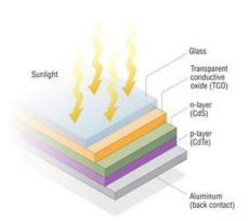
that result in total opacity. In other words, light cannot pass through the films, and they act essentially as mirrors. Opaque conducting films may be used as the **back contact** to the solar cell.
