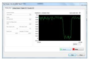
A to D) conversion. You can use Max to observe the voltage signal and determine whether or not, when you block the light, the voltage drops according to what you'd expect. Make sure you use RSE for the input configuration. If you see a signal within Max, you can optimize it through alignment.
