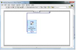
(at right) in frame #2. When configuring the writing of the file, please establish a "Data" folder within your Team X folder, and direct LabVIEW to use that folder when storing files. To determine if the data has been written to the file correctly, exit LabView and open/inspect the contents of the file with Notepad, the resident Windows text editor.
