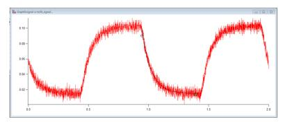
wheel has just blocked the beam. Place the 2<sup>nd</sup> (square) cursor near the bottom of the "run-out", just before the time when the chopper unblocks the beam. Go to Analysis, then choose Quick Fit
