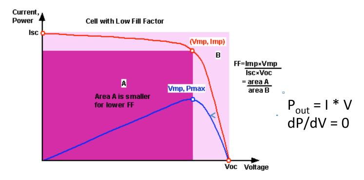
Graph of cell output current (red line) and power (blue line) as function of voltage. Also shown are the cell short-circuit current ( $I_{sc}$ ) and open-circuit voltage ( $V_{oc}$ ) points, as well as the maximum power point ( $V_{mp}$ ,  $I_{mp}$ ). Click on the graph to see how the curve changes for a cell with low FF.
