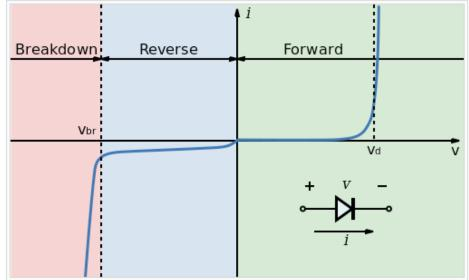
Figure 5: I–V characteristics of a p–n junction diode (not to scale—the current in the reverse region is magnified compared to the forward region, resulting in the apparent slope discontinuity at the origin; the actual I–V curve is smooth across the origin).
