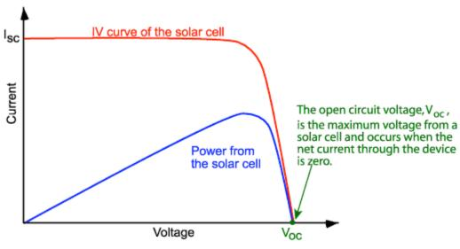
An equation for  $V_{oc}$  is found by setting the total current equal to zero, giving:
