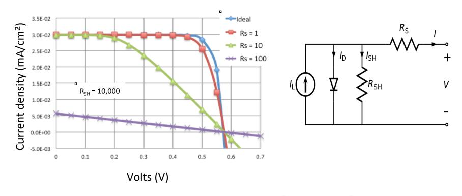
Diode equation with R<sub>S</sub> and R<sub>SH</sub>:
