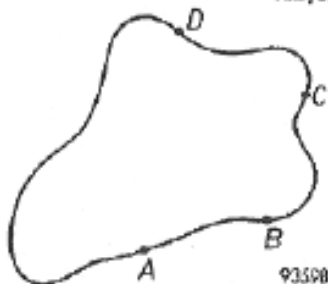
Fig. 3. A sample of arbitrary shape with four small contacts at arbitrary places along the circumference which, according to this paper, can be used to measure the specific resistivity and the Hall effect.
