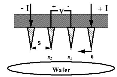
$$R = \int_{x_1}^{x_2} \rho \frac{dx}{2\pi xt} = \int_{x_2}^{2s} \rho \frac{dx}{2\pi xt} = \frac{\rho}{2\pi t} (\ln x) \Big|_{x_2}^{2s} = \frac{\rho}{2\pi t} \ln 2$$
