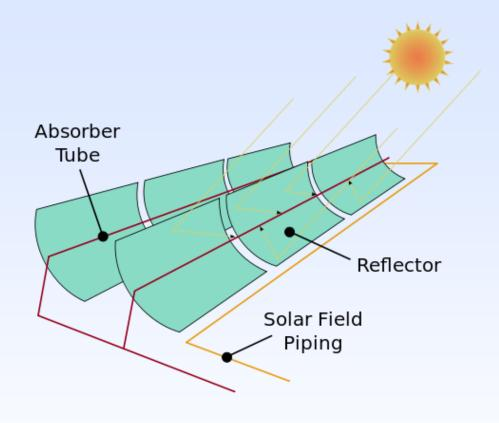
Absorber tubes contain a synthetic oil, and heat to > 400 °C by sunlight focused to ~75x standard sunlight. The heated oil then transfers heat to boil water, generate steam, and power the Rankine cycle steam turbine to generate electricity. Note that the troughs do not require 2-D tracking.
