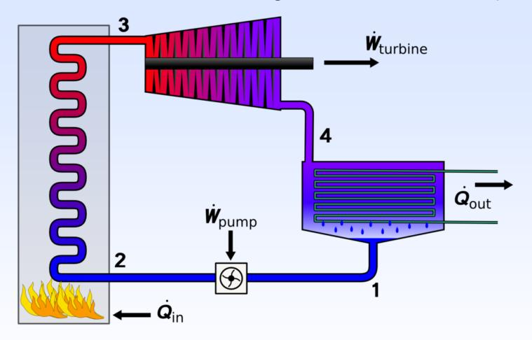
Diagram showing the basic layout of a Rankine cycle; Fluid is pumped to high pressure going from state 1 to 2. Heat is added in the boiler by the burning of fuel (although heat can be added by any method) boiling the fluid to state 3. The vapour expands through the turbine dropping significantly in pressure and temperature to state 4. Finally the vapour is condensed back to a liquid and fed back in the pump.
