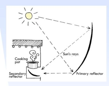
Focusing the Sun's rays onto a small surface area concentrates the intensity. These cookers can routinely reach ~300 °F.
