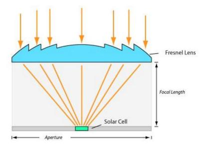
Named after the French physicist, comprises several sections with different angles; reduced weight and thickness compared to standard lens. Possible to achieve short focal length and large aperture while keeping the lens light. Constructed in a shape of a circle to provide a **point focus** with concentration ratios of around 500, or cylindrical shape to provide line focus with lower concentration ratios.
