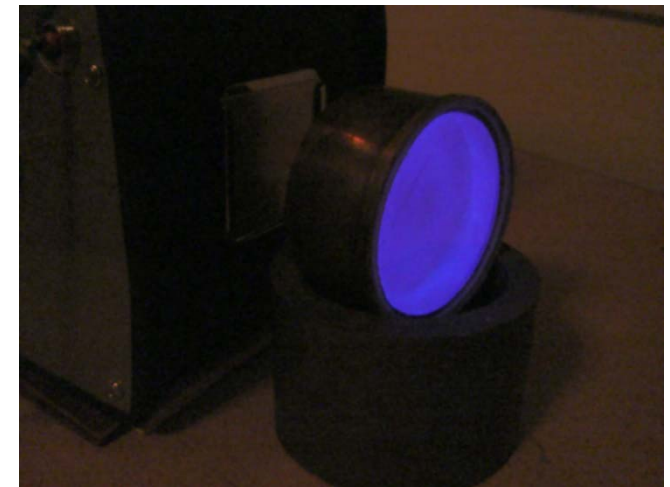
NaI:Tl emission following exposure to a \sim 300 R / hr x-ray field.
