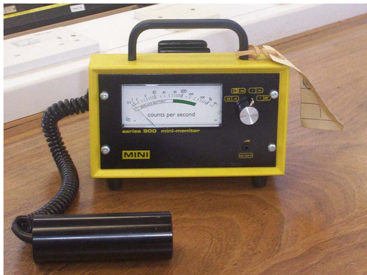
Geiger counter (based on Geiger-Müller tube)
