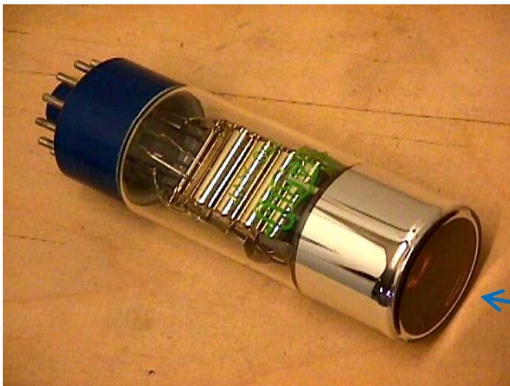
Typical PMT (end-on) detector.
