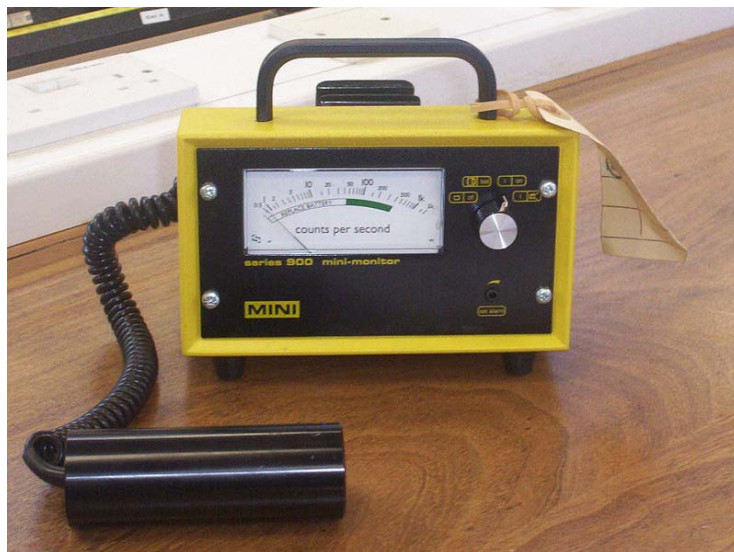
Geiger counter (based on Geiger-Müller tube)
