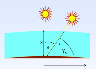
Therefore, on Jan. 30 at 1 pm, assuming clear weather: AM = 1.97. How about June 21, at noon? In that case,  $\gamma_s = 70.3^{\circ}$ , so that AM = 1.06.
