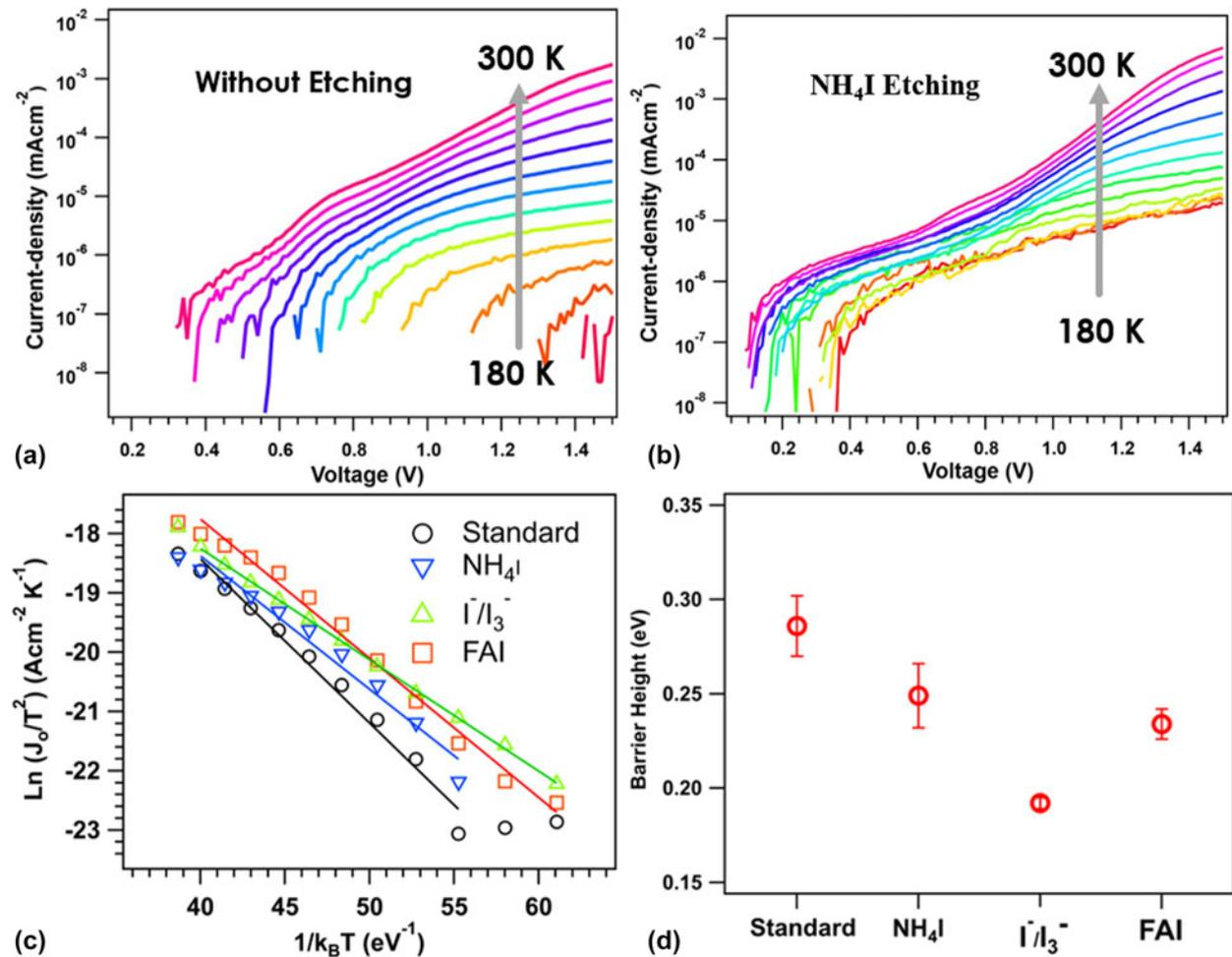
**Figure 8:** Temperature-dependent current–voltage ( $J-V-T$ ) characteristics of CdTe devices (a) without etching and (b) etching with  $NH_4I$  solution. (c) Plots of  $\ln(J_0/T^2)$  versus  $1/k_B T$  for standard and  $NH_4I$ ,  $I^-/I_3^-$ , and FAI etching and (d) values of back barrier height for standard and etched devices.
