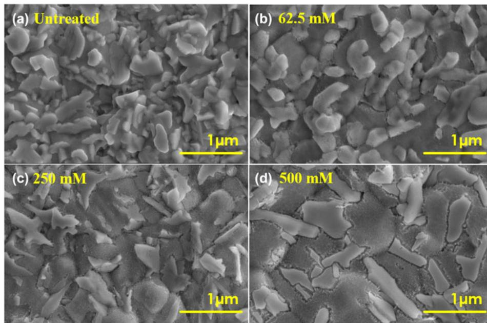
**Figure 6:** Surface topography of (a) standard CdTe surface and CdTe surface etched with FAI solution of concentrations: (b) 62.5 mM, (c) 250 mM, and (d) 500 mM. The CdTe films were annealed for 10 min at 150 °C before rinsing with 2-propanol in air environment.
