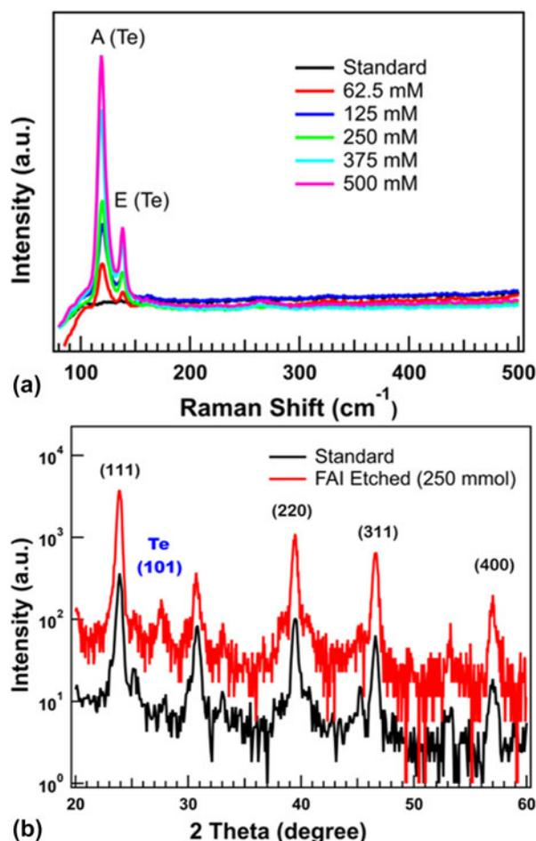
**Figure 5:** (a) Raman spectra of CdTe surface etched with various concentrations of FAI solution and (b) XRD patterns of standard and FAI-etched CdTe films.
