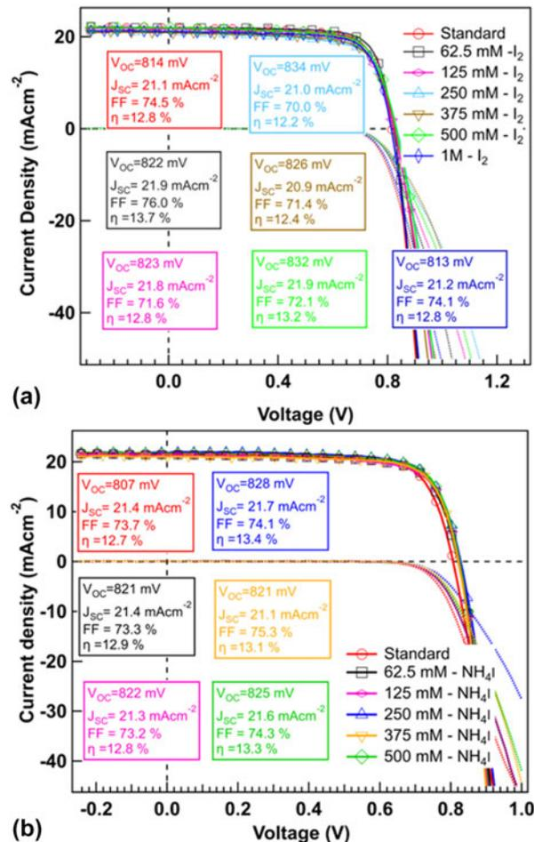
**Figure 3:** Typical  $J$ - $V$  characteristics of CdTe solar cells with (a) iodine and (b)  $NH_4I$  etching of various concentrations.
