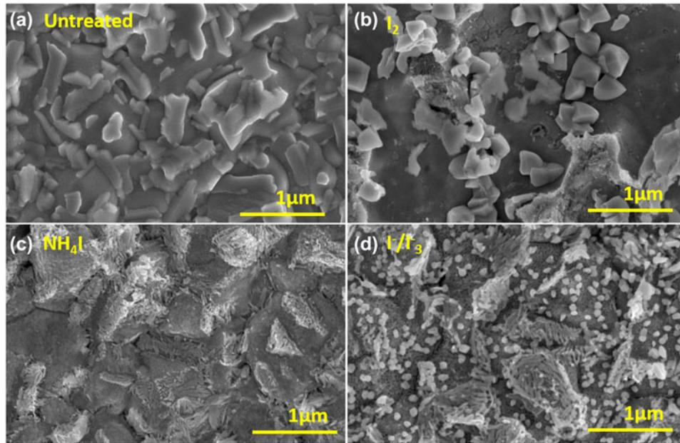
**Figure 2:** SEM images of CdTe thin films after etching with various iodine compounds: (a) untreated, (b) iodine ( $I_2$ ), (c) ammonium iodide ( $NH_4I$ ), and (d) mixed  $I^-/I_3^-$  solutions.
