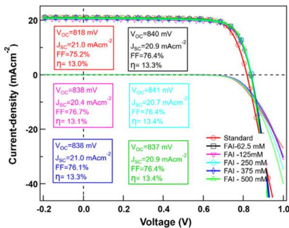
**Figure 7:** Current density versus voltage ( $J$ - $V$ ) characteristics of standard and FAI-treated cells.
