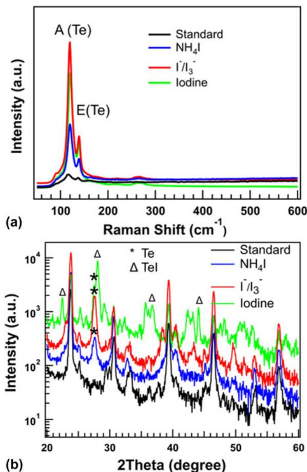
**Figure 1:** (a) Raman spectra and (b) XRD patterns of CdTe thin films after etching with iodine (I<sub>2</sub>), ammonium iodide (NH<sub>4</sub>I), and mixed I<sup>-</sup>/I<sub>3</sub><sup>-</sup> solutions. The peaks marked by \* at 27.6° are for Te (101) (PDF #97-002-3060) and peaks marked by Δ indicate Tel β-phase (PDF #97-000-0108).
