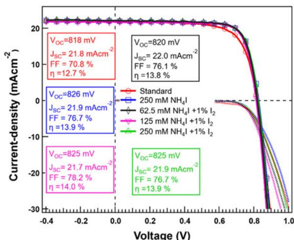
Figure 4: Typical *J-V* characteristics of CdTe solar cells with I<sup>-</sup>/I<sub>3</sub><sup>-</sup> etching of various concentration.
