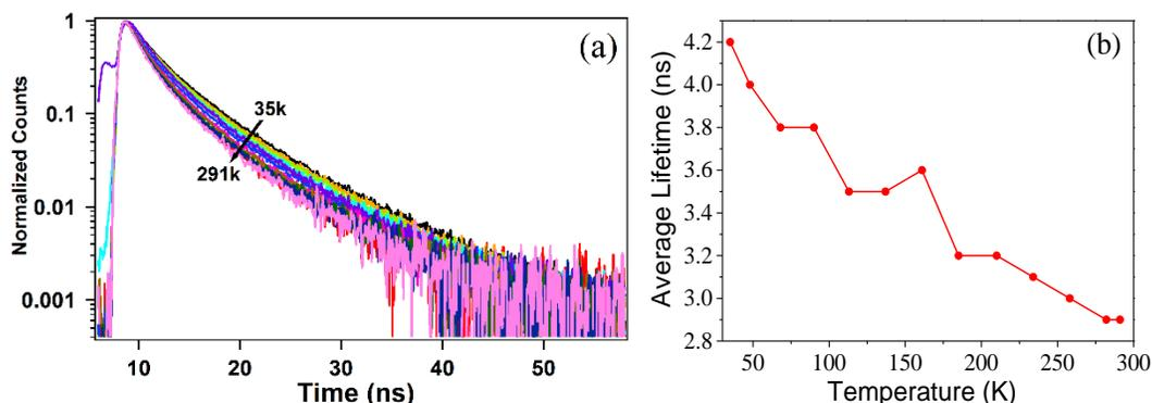
Figure 6. (a) Temperature-Dependent TRPL for the carbon dot sample from 35 K to 291K. (b) Estimations of average carrier lifetime from bi-exponential fits for the data.
