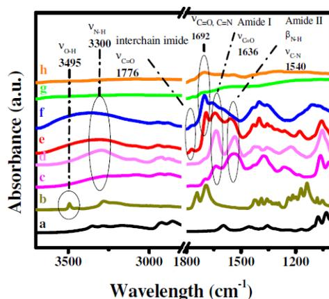
Figure 8. FTIR spectra of (a) ethanolamine, (b) citric acid, (c) CNP180, (d) PL-CNP180, (e) CNP230, (f) CNP300, (g) CNP400 and (h) ox-CNP400. Peaks that correspond to functional groups mentioned in the text are noted and identified. (The abbreviations used are: CNP, Carbon nanodot;  $\nu$ , stretching;  $\beta$ , in plane bending.)<sup>7</sup>
