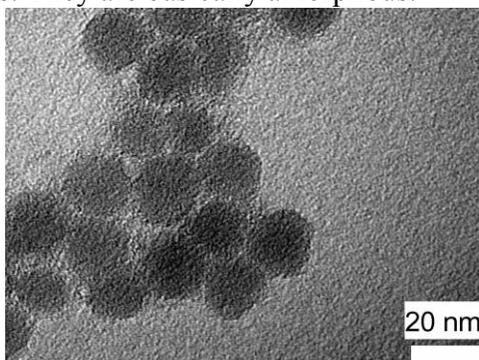
Figure 1. Transmission Electron Microscope (TEM) image of carbon dots.
