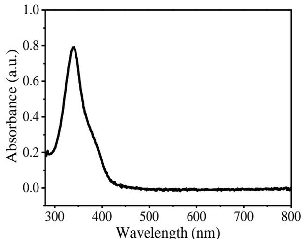
Figure 2. UV-Vis spectrum of carbon nanodots
