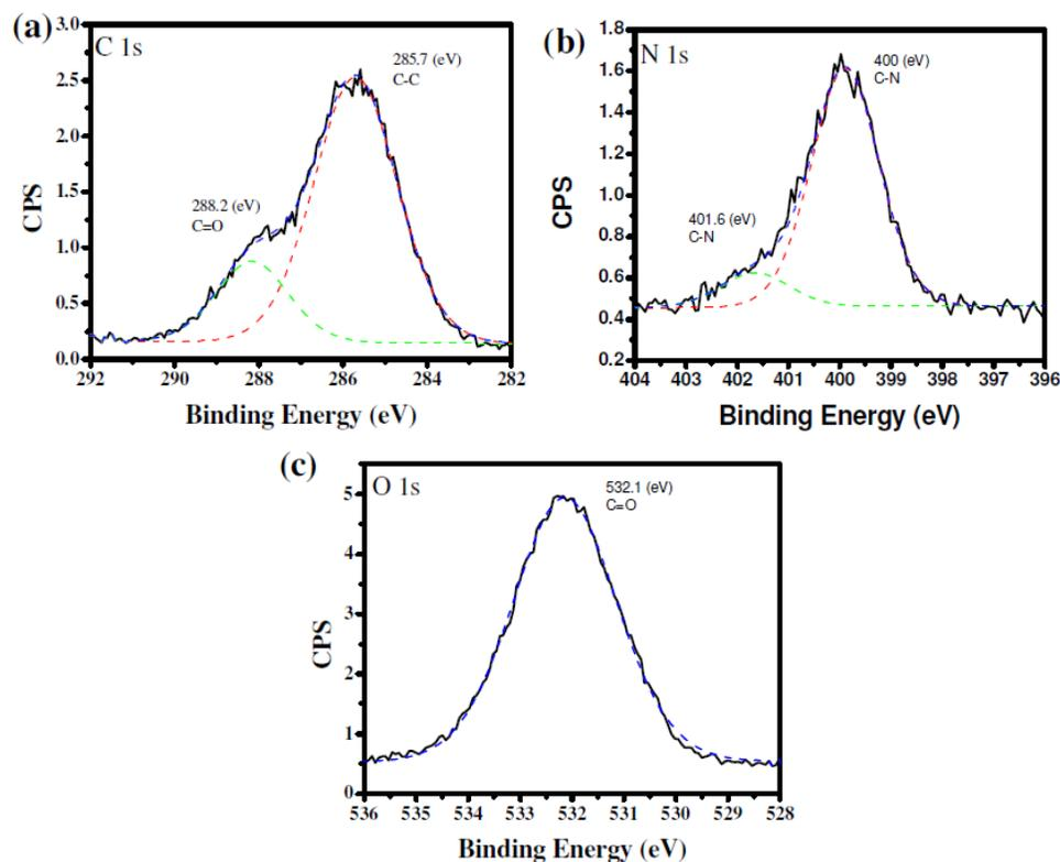
Figure 7. XPS spectra of carbon dots (a) C 1s, (b) N 1s and (c) O 1s. Full and dashed lines represent the data recorded and the fitted curves.<sup>7</sup>
