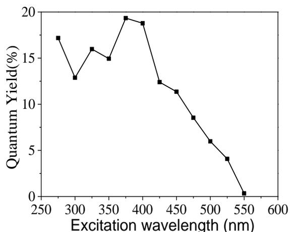
Figure 4. Excitation dependent Photoluminescence Quantum Yield of carbon nanodots
