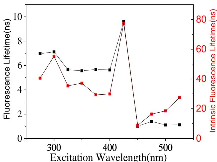
Figure 5. Excitation dependent photoluminescence Lifetime of PVA (Polyvinyl alcohol) dispersions of Carbon nanodots.
