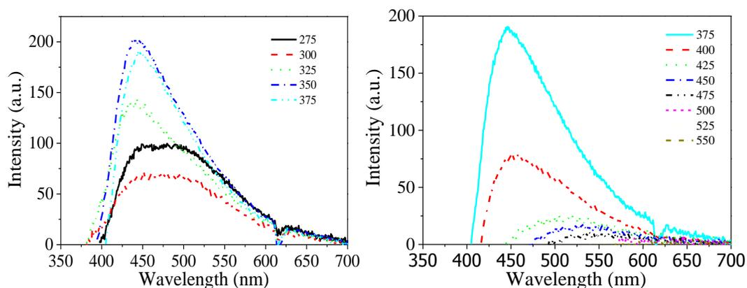
Figure 3. Excitation independent(Left) and dependent(Right)photoluminescence spectra of PVA (Polyvinyl alcohol) dispersions of Carbon nanodots
