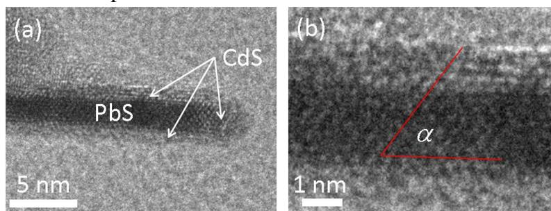
**Figure 3.** (a) HRTEM image showing atomically sharp interfaces between the PbS core and the CdS shell. (b) Zoomed-in HRTEM image showing the similar crystal structure of the CdS shell as the PbS core. The lines are to guide the eyes to the array of ions, making the angle  $\alpha$  unique to {110} facet as mentioned earlier.<sup>14</sup>
