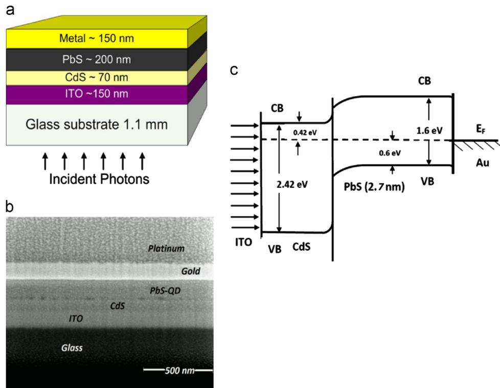
**Fig. 1.** (a) Schematic of the PbS QD/CdS heterojunction solar cell. (b) Cross-sectional scanning electron microscopy (SEM) of the PbS QD/CdS junction solar cell illustrated in (a). (c) Schematic of the energy band diagram of an ITO/CdS/PbS-QD/Au solar cell.
