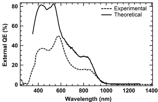
Fig. 3. External quantum efficiency spectrum of the PbS-QD solar cell featured in Fig. 2 from both theoretically and experimentally obtained data. In the theoretical curve, charge collection contribution from both CdS and PbS-QD layers are considered and recombination losses are neglected.
