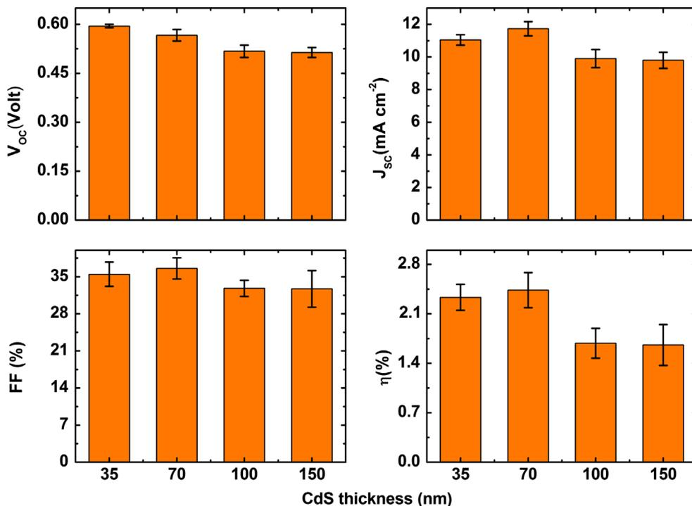
Fig. 5. Dependence on window layer thickness of the performance of PbS-QDs solar cells. Six devices for each CdS thickness (35, 70, 100 and 150 nm) were fabricated on a single substrate by depositing a PbS-QD film of thickness  $\sim 200$  nm. The PbS QD diameter used in these studies was  $\sim 2.78$  nm, corresponding to the first exciton peak at 816 nm (1.52 eV).
