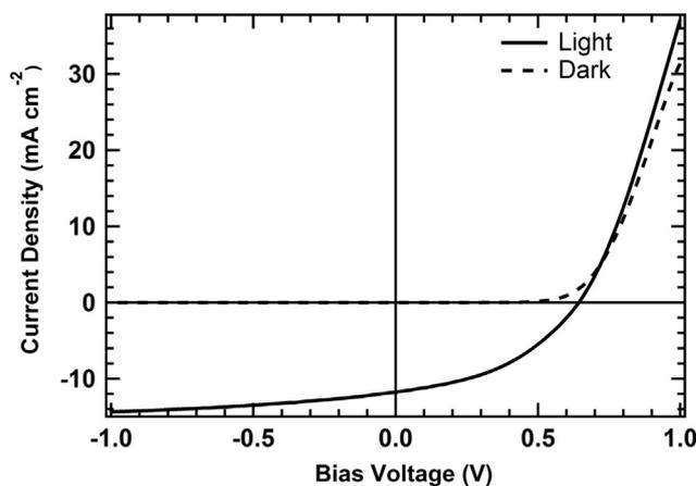
Fig. 2. Current–voltage (*I*–*V*) characteristics of a CdS/PbS-QD heterojunction solar cell recorded in the dark and under 100 mW·cm<sup>-2</sup> simulated AM1.5 illumination. The device was assembled using ~200 nm thick EDT treated PbS-QD film deposited from ~2.7 nm diameter QDs, ~70 nm thick CdS film and gold contact.  $V_{OC}$ ,  $J_{SC}$ , FF and PCE of this cell were 638 mV, 12.0 mA·cm<sup>-2</sup>, 43.5% and 3.3% respectively.
