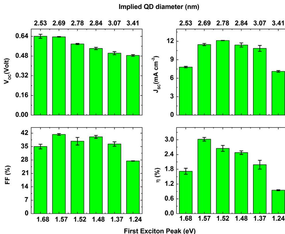
Fig. 4. Dependence of  $V_{OC}$ ,  $J_{SC}$ , FF and PCE on the diameter and effective band gap energy (the first exciton peak,  $E_g$  in eV) of PbS-QDs. All solar cell devices were assembled using  $\sim 200$  nm thick EDT-capped PbS-QD film deposited onto  $\sim 70$  nm thick CdS. Diameters of the QDs are based on the first exciton peak values as measured in solution [34, 35].
