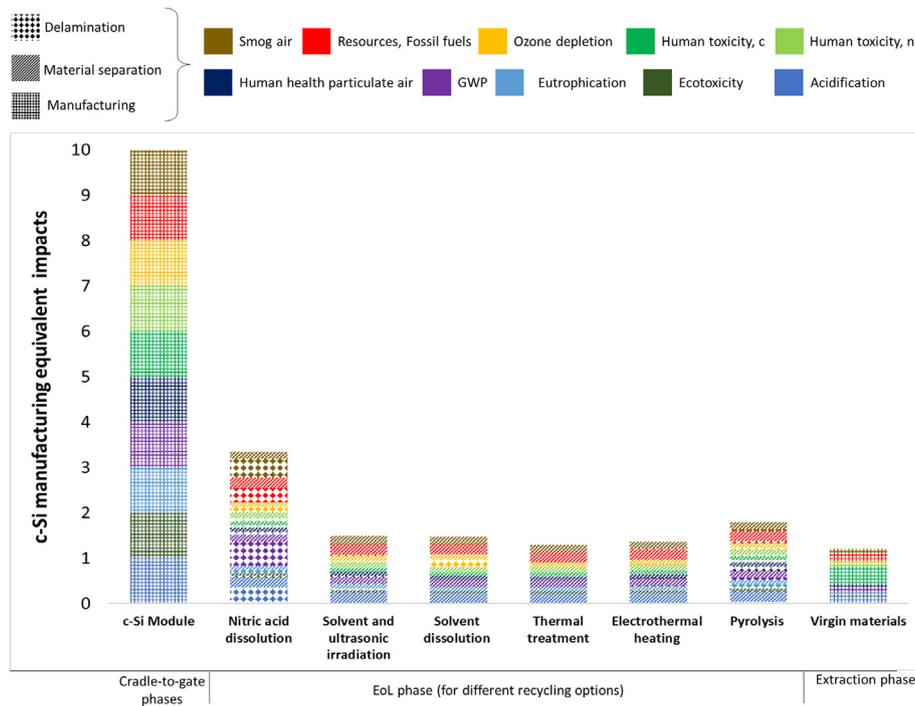
**Fig. 4.** Comparison of impact results for c-Si delamination with material separation (chemical etching) incorporated into each method and normalized to c-Si manufacturing. Within each impact category, the impact (per m<sup>2</sup> of panel recycled) from each process was divided by the impact from c-Si manufacturing. For c-Si the bar height is unity for each impact category. For ten impact categories, the total impact for c-Si is given as ten units.
