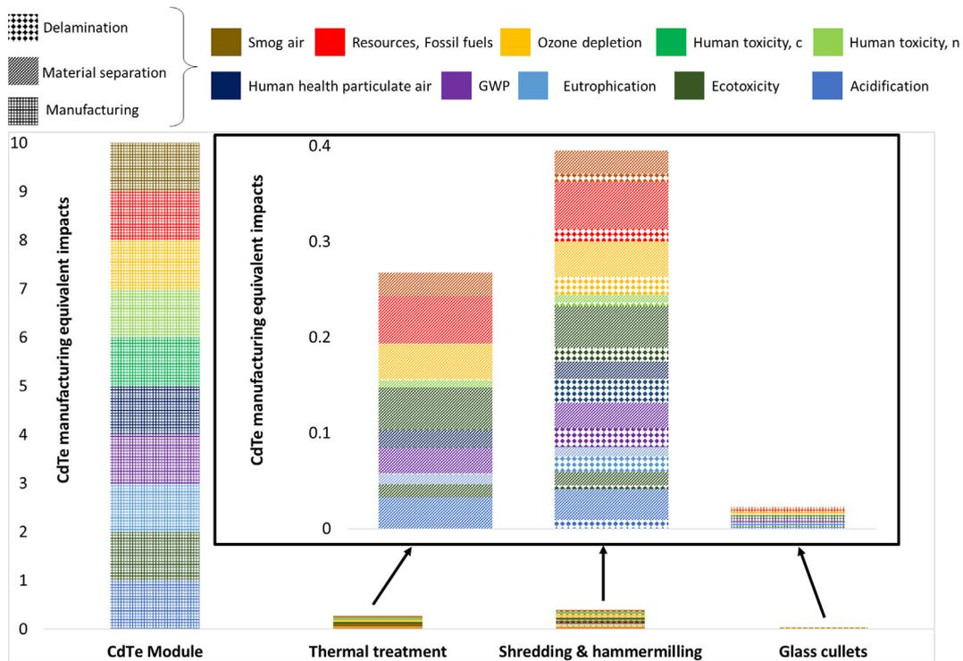
**Fig. 5.** Comparison of impact results for CdTe delamination with material separation impacts incorporated and normalized to CdTe manufacturing. Within each impact category, the impact (per m<sup>2</sup> of panel recycled) from each process was divided by the impact from CdTe manufacturing. For thin films the bar height is unity for each impact category. For ten impact categories, the total impact for CdTe is given as ten units.
