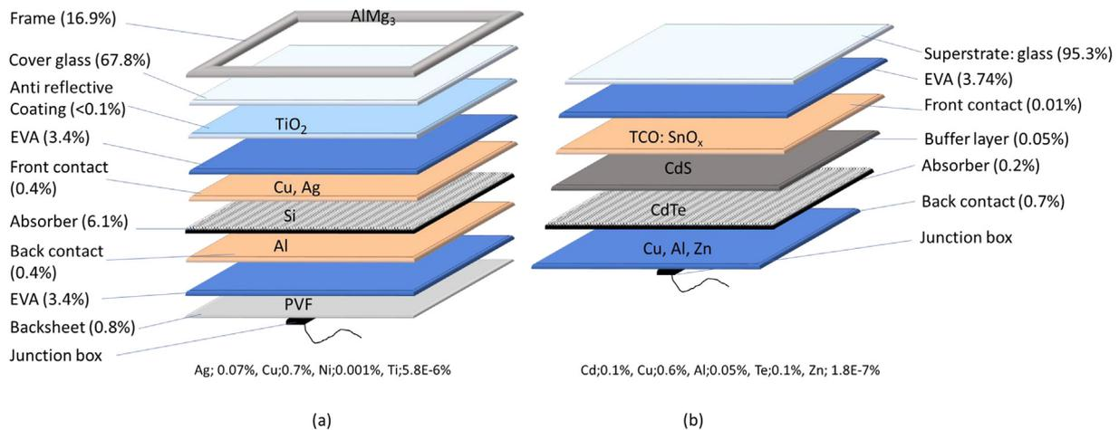
Fig. 1. Typical PV structure of (a) c-Si and (b) CdTe PV panels with percentage mass compositions. The percentage mass compositions are an average of data from six different sources (Bekkelund, 2013; Domínguez and Geyer, 2017; Frischknecht et al., 2015; Jungbluth et al., 2012; Sander et al., 2007a, 2007b; Stolz et al., 2016). EVA: Ethylene Vinyl Acetate, TCO: Transparent Conducting Oxide, PVF: Poly Vinyl Fluoride.
