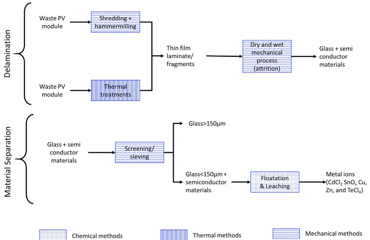
Fig. 3. Delamination and material separation methods for CdTe PV panels. Material inputs for each method are shown in Table 1.
