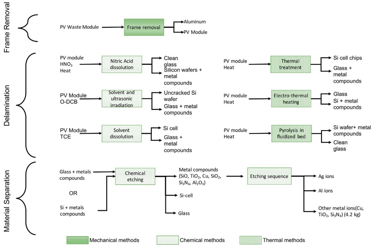
Fig. 2. Delamination and material separation methods for c-Si. Material inputs for each method are shown in Table 1.
