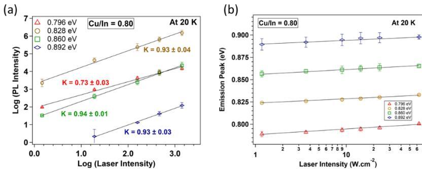
Figure 4. (a) Power law dependence for observed peaks and (b) emission peak vs. laser intensity in CuInSe<sub>2</sub> film with Cu/In = 0.80.
