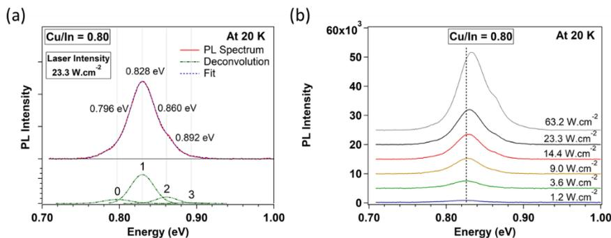
**Figure 3.** (a) PL spectrum along with multi-gaussian fits and (b) laser excitation dependent PL of CuInSe<sub>2</sub> films with Cu/In = 0.80.
