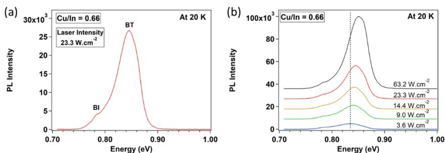
**Figure 1.** PL spectra of CuInSe<sub>2</sub> film with Cu/In = 0.66 taken at 20 K (a) showing BT and BI band (b) for various intensities of laser.
