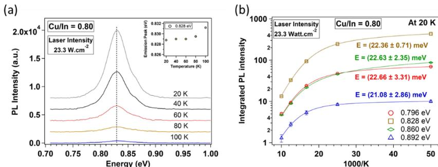
**Figure 5.** (a) Temperature dependent PL spectra and (b) temperature dependence of PL intensity of observed peaks for the CuInSe<sub>2</sub> film with Cu/In = 0.80.
