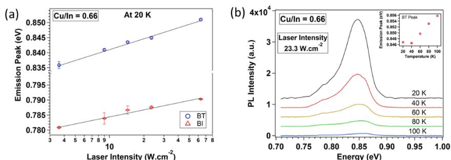
**Figure 2.** (a) Peak emission vs. laser intensity at 20 K and (b) temperature dependence of PL intensity of CuInSe<sub>2</sub> film with Cu/In = 0.66.
