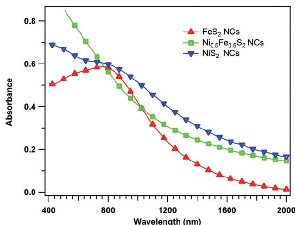
Fig. 4 UV-Vis-NIR absorption spectra of Ni-alloyed ( $\text{Ni}_x\text{Fe}_{1-x}\text{S}_2$ ) iron pyrite NCs with different material composition pure  $\text{FeS}_2$  NCs,  $\text{Ni}_{0.5}\text{Fe}_{0.5}\text{S}_2$  NCs and  $\text{NiS}_2$  NCs solution dispersed in chloroform. Symbol point spacing is greater than the actual data point spacing.
