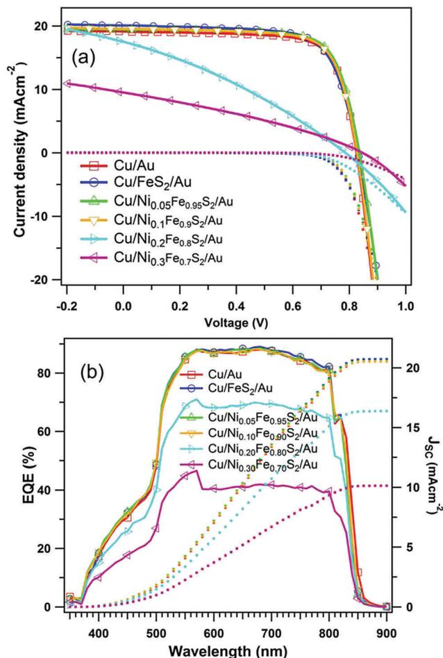
Fig. 6 Device performance when  $\text{Ni}_x\text{Fe}_{1-x}\text{S}_2$  NCs films were used as interface layers in CdTe solar cells: (a)  $J$ - $V$  characteristics with AM 1.5G simulated irradiance, and (b) external quantum efficiencies (EQEs).
