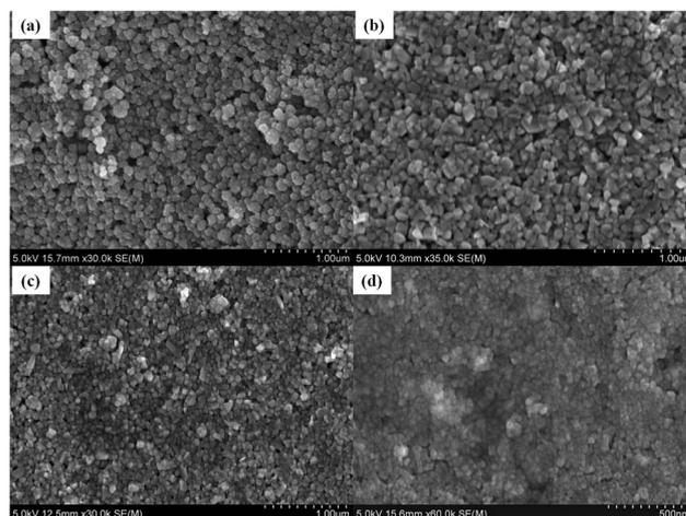
Fig. 3 Scanning electron microscopy (SEM) images of Ni-alloyed iron pyrite nanocrystals with different material compositions (a)  $\text{FeS}_2$  NCs (b)  $\text{Ni}_{0.1}\text{Fe}_{0.9}\text{S}_2$  NCs (c)  $\text{Ni}_{0.2}\text{Fe}_{0.8}\text{S}_2$  NCs (d)  $\text{Ni}_{0.5}\text{Fe}_{0.5}\text{S}_2$  NCs. The particle size of the alloyed NCs decreases as Ni fraction increases.
