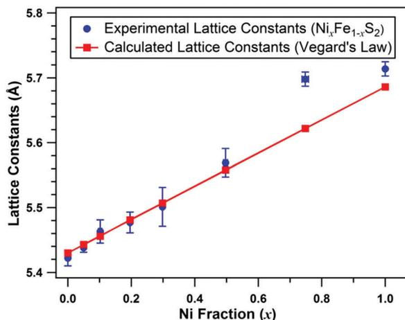
Fig. 2 Lattice constants for Ni-alloyed iron sulfide ( $\text{Ni}_x\text{Fe}_{1-x}\text{S}_2$ ) pyrite nanocrystals for seven different compositions. The experimental lattice constant values agree closely with the predicted lattice constant values (Vegard's law) up to the Ni fraction  $x = 0.5$ , and it is slightly too high for the highest concentrations of Ni.
