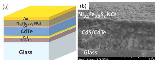
Fig. 5 Device structure of CdTe solar cell using  $\text{Ni}_x\text{Fe}_{1-x}\text{S}_2$  as back contact material (a) schematic diagram of the device structure (b) cross-sectional SEM image of CdS/CdTe solar cells with  $\text{Ni}_{0.1}\text{Fe}_{0.9}\text{S}_2$  NCs as interface layer.
