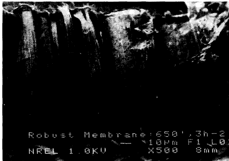
Figure 1. Robust array of carbon nanotubes (aspect ratio ca. 7000) formed at 600 °C.
