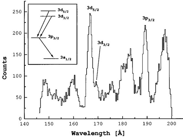
FIG. 1. A partial channel-plate spectrum taken at an observing position close to the exciter foil. The inset shows the relevant transitions used in the ANDC analysis. All transitions in the spectrum have been identified.
