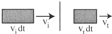
From the diagram,  $T = P_t/P_i = |F|^2 v_t / |A|^2 v_i$ , where  $P_i$  is the probability of finding the incident particle in the box corresponding to the time interval  $dt$ , and  $P_t$  is the probability of finding the transmitted particle in the associated box to the *right* of the barrier.
