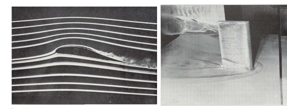
Figure 2.4 Smoke photograph of the low-speed flow over a Lissaman 7769 airfoil at 10° angle of attack. The Reynolds number based on chord is 150,000. This is the airfoil used on the Gossamer Condor man-powered aircraft. (The photograph was taken in one of the Notre Dame University smoke tunnels by Dr. T. J. Mueller, Professor of Aerospace Engineering at Notre Dame, and is shown here through his courtesy.)
