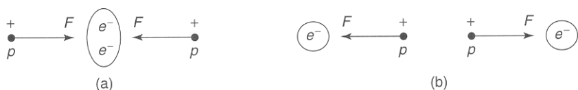
FIGURE 5.1: Schematic picture of the covalent bond: (a) Symmetric configuration produces attractive force. (b) Antisymmetric configuration produces repulsive force.
