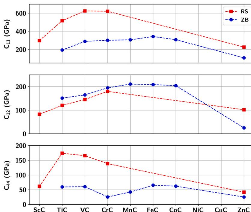
**Fig. 4.** Independent elastic constants ( $C_{11}$ ,  $C_{12}$ ,  $C_{44}$ ) shown for all the stable/metastable compounds in the rocksalt structure (RS) and zincblende structure (ZB). Symbols represent calculated values, whereas the lines represent interpolations plotted to highlight general trends.
