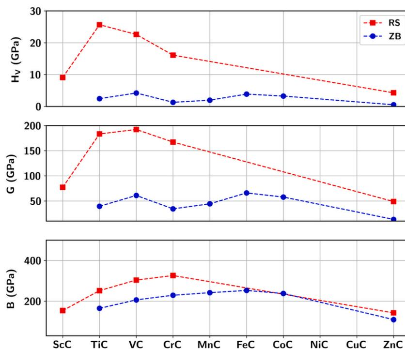
**Fig. 5.** Correlation of Vickers hardness ( $H_v$ ), shear modulus ( $G$ ), and bulk modulus ( $B$ ) with increasing group number across all stable/metastable 3d TMCs in the rocksalt structure (RS) and zincblende structure (ZB). Symbols represent calculated values, whereas the lines represent interpolations plotted to highlight general trends.
