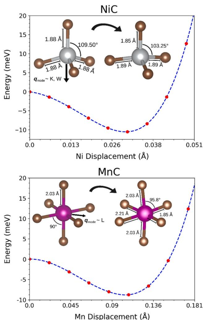
**Fig. 1.** Illustration of the energy landscapes, modulated along instabilities at high-symmetry points according to phonon dispersion calculations, for NiC (top) and MnC (bottom) in the zincblende and rocksalt structures respectively. Insets show local bonding configurations (tetrahedra and octahedra) before and after application of distortions. For the latter, bond lengths and angles corresponding to a minimum in energy are listed.
