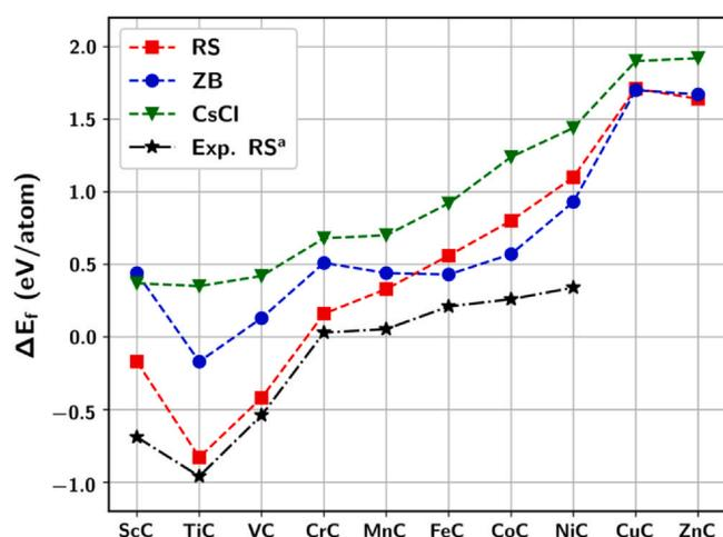
**Fig. 3.** Calculated formation energies of all 3d transition metal carbides in the rocksalt structure (RS), zincblende structure (ZB), and cesium chloride structures (CsCl). Symbols represent calculated values, whereas the lines represent interpolations plotted to highlight general trends. (a): Experimental formation energies are from Ref. [40].
