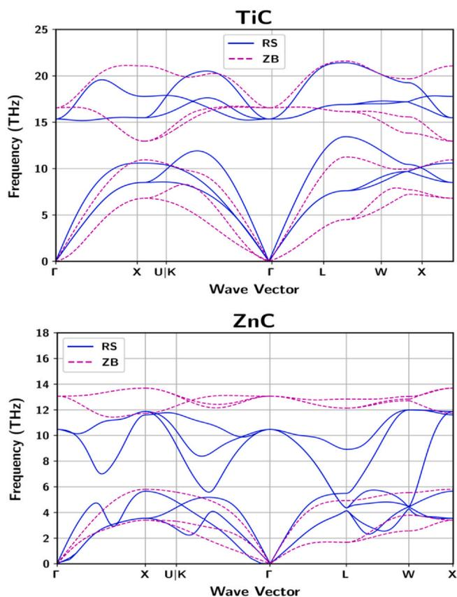
Fig. 6. Phonon dispersion curves for TiC and ZnC, each of which represents extrema in the valence electron concentration of all stable compounds. To illustrate dynamic differences arising from varying structural factors, individual curves are plotted for the rocksalt (RS) and zincblende (ZB) structures.
