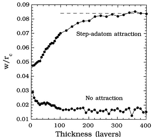
FIG. 3. Mound angle ratio  $w/r_c$  as a function of film thickness with step-adatom attraction ( $R' = 10$ ) and without step-adatom attraction ( $R' = 1$ ).
