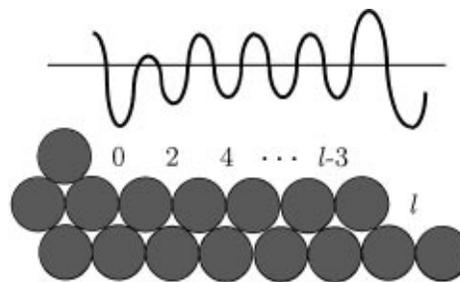
FIG. 1. Diagram showing stepped bcc/fcc (100) surface with slope  $m$  (terrace width  $l = 1/m$ ) and straight step edges along the (001) axis (side view). Even sites correspond to fourfold-hollow sites on terrace. Also shown is a schematic of the potential surface showing decreased potential barrier due to step-adatom attraction near the ascending step along with a possible step barrier at the descending step.
