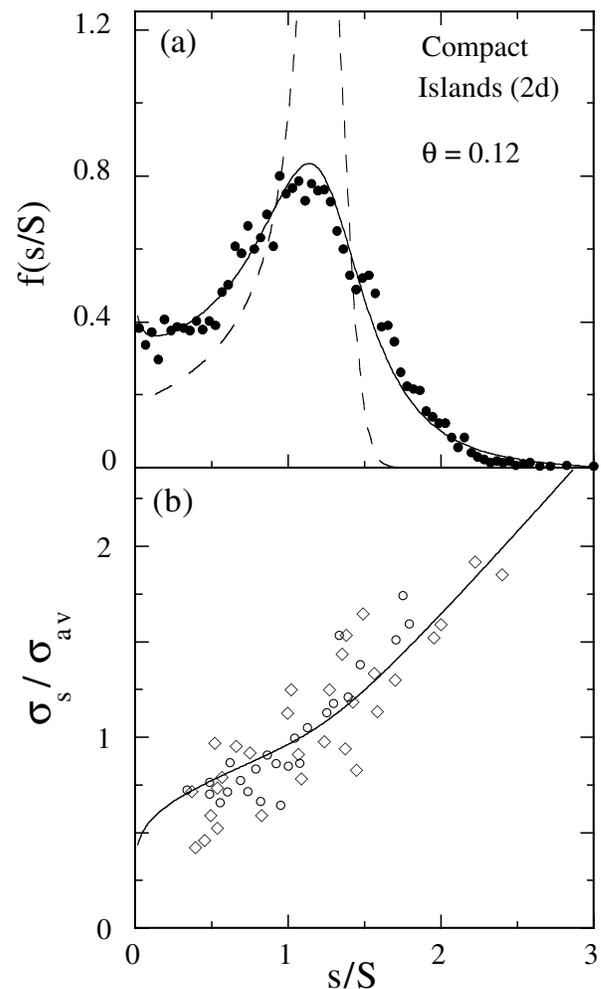
FIG. 3. Same as Fig. 2 but for compact islands ( $d_f = 2$ ). Open symbols in (b) are experimental results from [8] for Cu/Co on Ru(0001) (diamonds) and for Ag/Ag(100) (circles).
