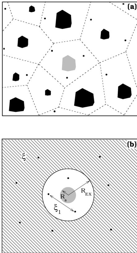
FIG. 1. Schematic diagram showing (a) two-dimensional islands with Voronoi cells (b) corresponding exclusion zone geometry.
