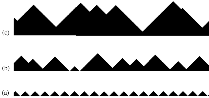
Fig. 2. Sequence of configurations in ghost-particle model (bottom to top) corresponding to (a) starting configuration, (b) 1.25 layers, and (c) 3.75 layers.
