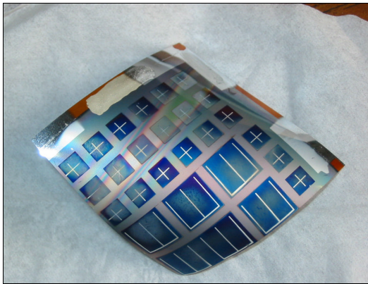
Fig 3.: Triple junction a-Si cells on Mo-coated Kapton VN
