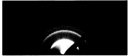
Figure 7 RHEED pattern of a device with VHF p-layer at the top, showing high volume fraction of microcrystalline phase in the p-layer.
