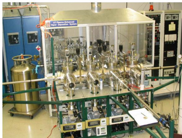
Fig. 2 Photo of UT's 9-chamber solar cell fabrication system.
