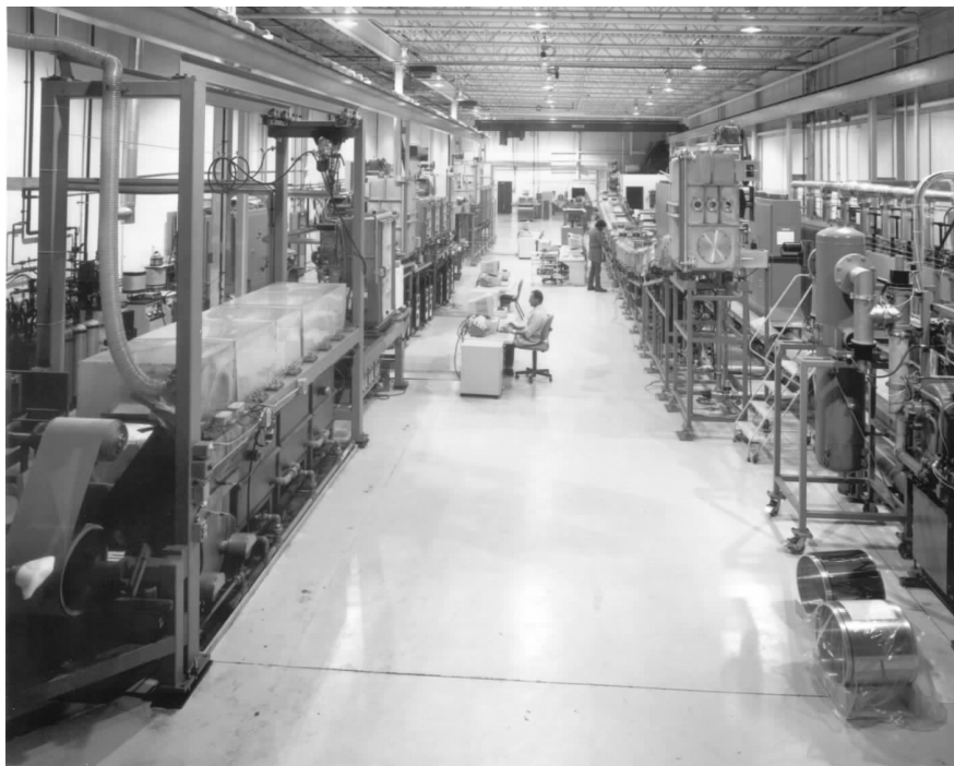
FIG. 27: A photograph of the Energy Conversion Devices, Inc. 2 MW plant showing all four front-end roll-to-roll machines for washing, back-reflector sputter deposition, PECVD deposition (right hand side) and TCO deposition. After Izu, et al. [186].
