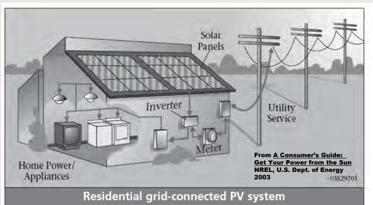
For a <u>grid-tied</u> system, back-up is already in place in the form of the utility company's grid
