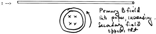
If the current in the wire is made to gradually increase as time passes, a current will be induced in the loop that flows (as viewed on this diagram)
