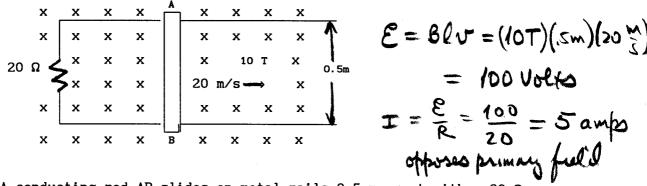
A conducting rod AB slides on metal rails 0.5 m apart with a 20  $\Omega$  resistor attached as shown above. The apparatus is in a uniform magnetic field of 10 T directed perpendicularly inward to the page. The rod is moving to the right at a speed of 20 m/s. What is the magnitude of the induced current? Is it clockwise or counterclockwise?
