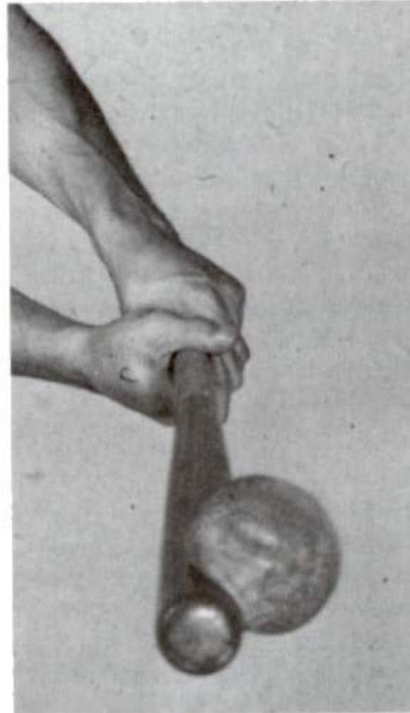
The collision of a ball with a bat collapses part of the ball.
